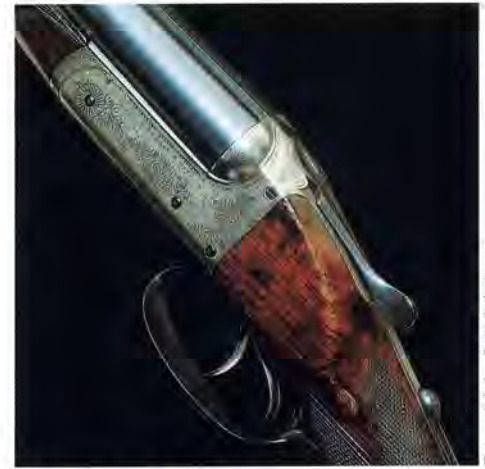
C-quality Purdey boxlock non-ejector .450/400 rifle no. 13963 – sold in 1891 to Lancashire-based industrialist Sir William Rylands.
