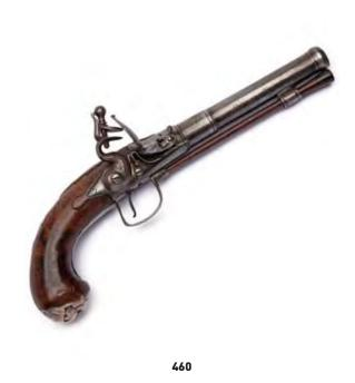
**A.670 FLINTLOCK FRENCH 1805 STYLE NAPOLEONIC SERVICE PISTOL SIGNED FRECONNET, no visible serial number,** circa 1810, with octagonal to round 8in. barrel, solid squared top-tang, flat bevel-edged lock with stepped and pointed tail and marked with a crown over 'S.E.' above the signature, iron pan, swan-necked cock, walnut half-stock, brass furniture including heavy pommel-cap and broad nose barrel-band, complete with nail-headed iron ramrod
