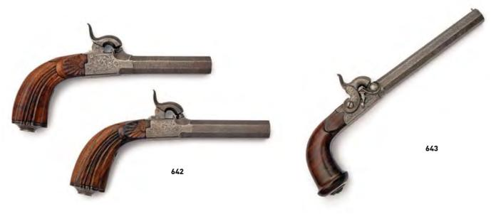
A PAIR OF 32-BORE RIFLED PERCUSSION CONTINENTAL BOXLOCK POCKET PISTOLS, UNSIGNED, no visible serial numbers, Belgian circa 1840, with etched damascus octagonal 3in. turn-off barrels (one frozen) rifled in eight grooves, squared boxlock central hammer actions with concealed automatic triggers and borderline and scroll engraving, fluted walnut grips with shell carved heads and sideways hinged moulded and engraved iron traps at heel £300-500
