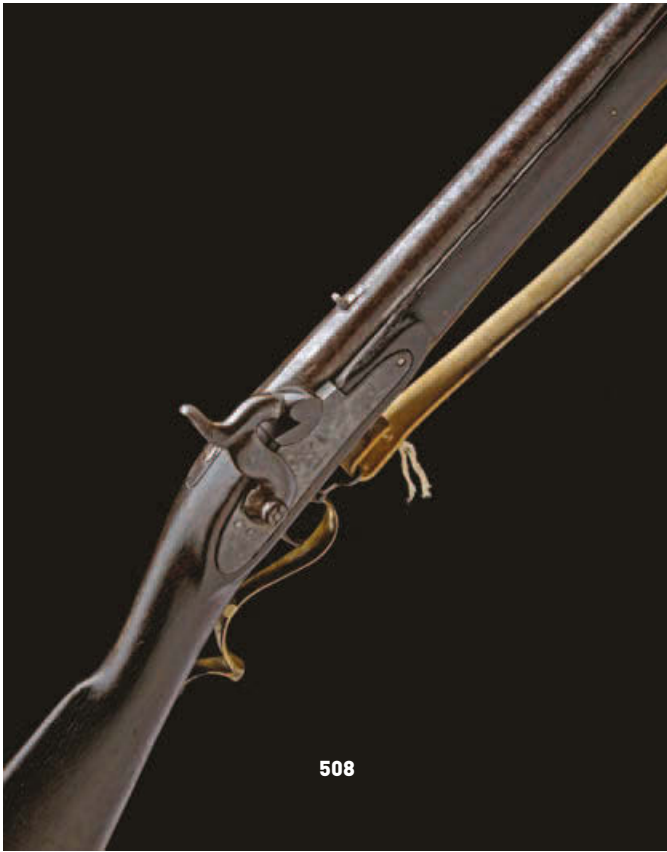
508 A .750 PERCUSSION EAST INDIA COMPANY TYPE 'C' PATTERN 1842 MUSKET, rack no. D72 , mid nineteenth century, with darkly stained round 39in. barrel, block fore-sight, fixed standing notch rear-sight, London proofs, knock-off breech with solid top-tang and rounded tip, flat semi-bevelled edge lock of flint form marked with the East India Co. rampant lion trademark and stamped with 'D5' below the nipple bolster, walnut full-stock stamped with 'D72' on the right side of butt and 'H104' (rubbed) on the right, along with various amateur applied farsi markings, brass furniture, the trigger guard bow with further farsi marks, three ramrod pipes and iron ramrod with squared shank behind the bun tip, fitted with a later buff leather sling £500-700
