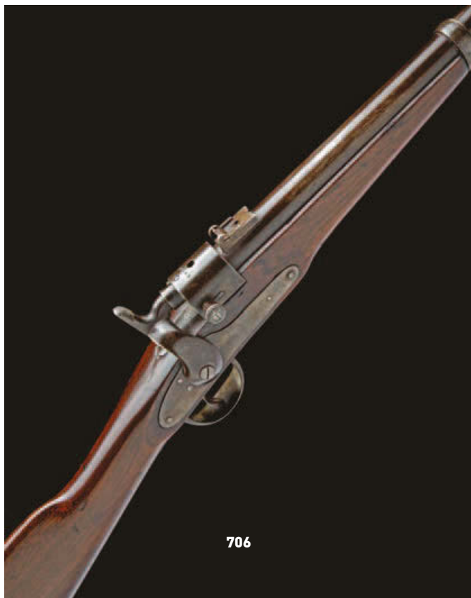
706 A .56-52 (RIMFIRE) MODEL 1864 JOSLYN BREECH-LOADING CARBINE OF THE AMERICAN CIVIL WAR, serial no 10455 , dated for 1864, with round tapering 22in. barrel, blade fore-sight, folding leaf rear-sight, pivoting breech-block marked on the rear face 'B.F. JOSLYN'S PATENT, OCTOBER 8TH 1861 JUNE 24TH 1862' and drilled with vent-hole, bar-action lock marked 'JOSLYN FIRE ARMS CO STONINGTON CONN.' and the date '1864', saddle-ring and bar to the left hand side and walnut half-stock (cracked through and well repaired behind lock) and fitted with iron furniture £700-900
